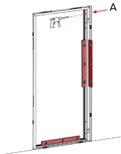
Fig. 14. Drilling the hole.
